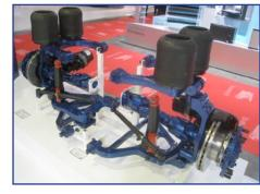
ned underbody, suspended with brackets. The steering angle with single wheel is 35 degrees.
