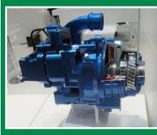
DIWA SmartNet and the air compressors. The DIWA automatic transmission was specifically developed for buses. Compared with its predecessor model, the DIWA.6 can save almost another 5% fuel. Apart from utili-
