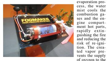
fire. The Fogmaker system includes a low concentration of AFFF to create an aqueous insulation film for the effective combustion suppression.
