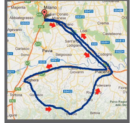
Ballasted at 5,260 kg (maximum curb weight is 5,300 kg), the VIP MidEuro traveled 308 kilometres from Milan to Passo del Penice and back via Piacenza (197 kilometres on the highway), consuming an average of one litre of diesel fuel every 7.89 km. Average travelling speed was 73 km/h.
