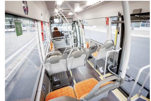
The panoramic windscreen with integrated destination display stretches right up into the roof, while the vehicle sides are extensively glazed and the belt line low. The overall effect is light and aesthetically pleasant. The driver's workplace is based on the cockpit of the new Mercedes-Benz Sprinter. There are such functional elements as the convex
